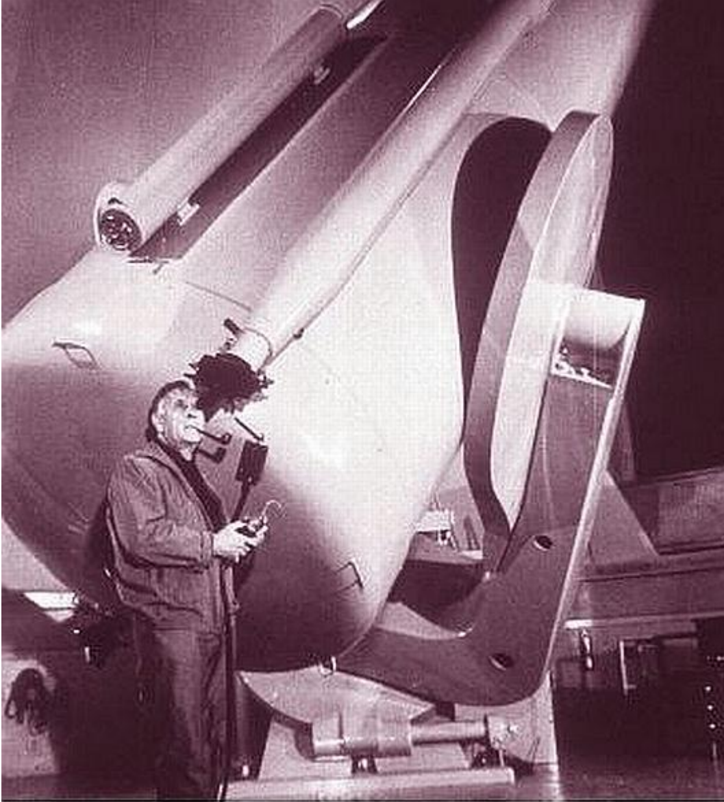
Dr. Hubble, the noted American astronomer, guiding the 48-inch Schmidt camera on Mount Palomar. Because of its wide-angle vision, this instrument has been able to complete in 7 years a photographic survey of the sky which would have taken the 200-inch Hale telescope 5,000 years to accomplish.
