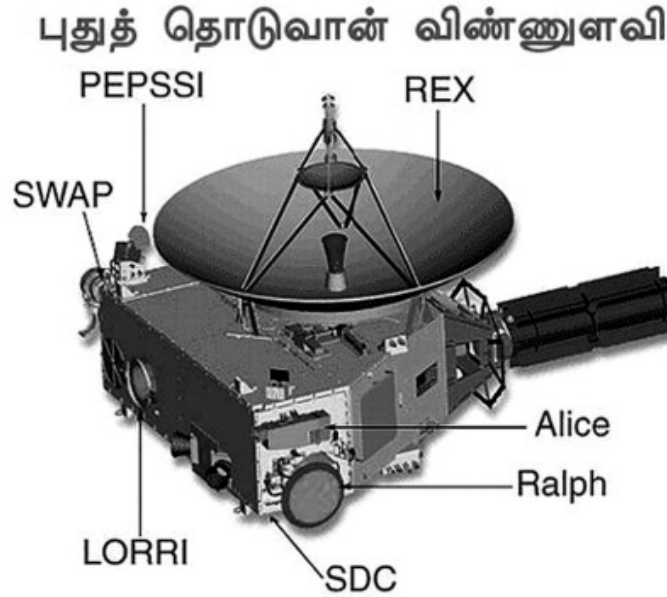
New Horizons Spacecraft and Instruments
